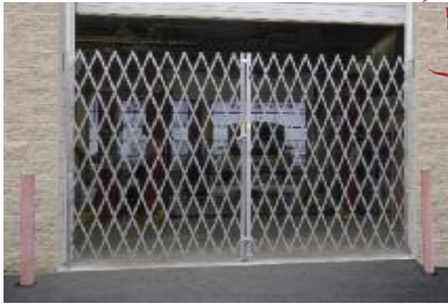
Heavy-Duty Pair Folding Gate Specifications: Galvanized finish. Heavy-duty 14 gauge steel u-channel webbing riveted back to back with zinc plated rivets. Heavy-duty 12 gauge steel 1-1/2" x 1-1/2" vertical angle frame. Solid steel casters. Padlock order separate.
