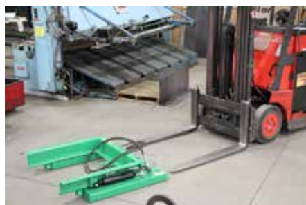
Step 1: Connect the Fork Lift Attachment and secure into place.
