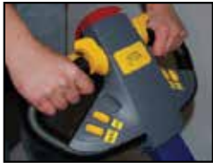
Curtis TM-1 Tiller head equipped with emergency reverse switch, electronic throttle, rocker switches, horn, and gas spring to automatically return head to upright position when not in use.
