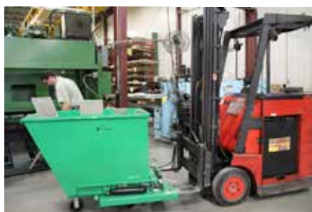
Step 2: Roll Mobile Hoppers to Fork Lift Attachment and engage secure latching system.
