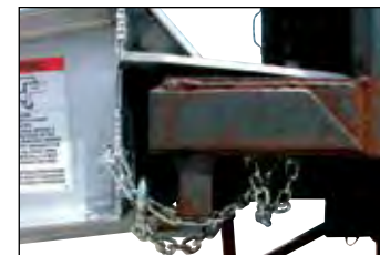
15" OVERLAP INTO TRAILER/BUILDING SAFETY CHAINS STANDARD
