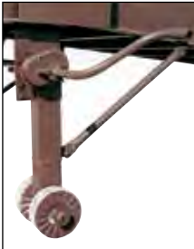
MANUAL HAND CRANK & 9" STEEL WHEELS
