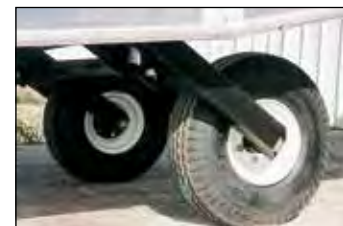
PNEUMATIC TIRES OPTION Service Range will be 40" to 66" model AY-PNTR
