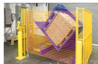
LIGHT CURTAINS: Provides a soft guarding across the front of the machine for additional protection
