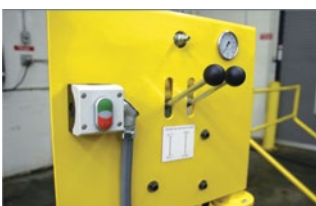
LEVERS: Basic control package will turn machine on/off, as well as clamp, un-clamp, and rotate
