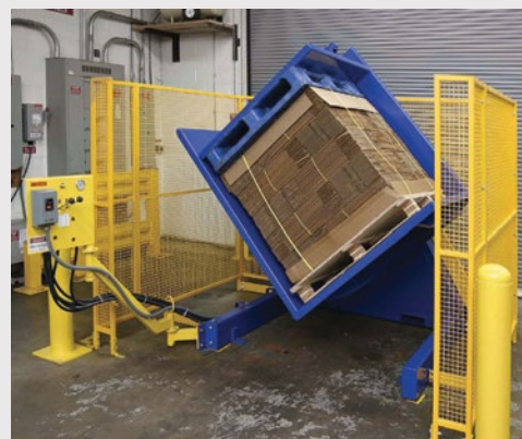
SAFELY TRANSFER CORRUGATE FROM A WOOD PALLET TO A PLASTIC PALLET
