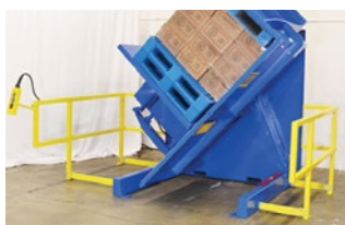
STANDARD MACHINE GUARDING: Provides protection from forklifts
