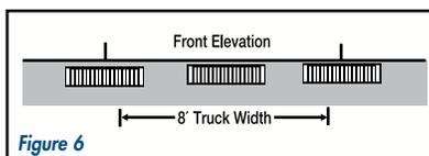
Overlapping reduces the spacing between each bumper to 4", and is applicable to any Durable laminated bumper model.
