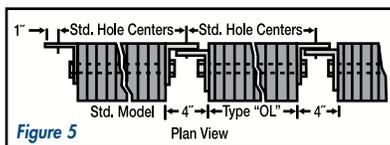
For an angled truck approach, spacing should be reduced to prevent a truck corner from contacting the dock between units.
