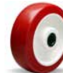
Poly-Tech® (NF) 350 - 1,200 lbs. Sleek, resilient wheels for sanitary use. They feature a non-marking, steam cleanable tread of red polyurethane mechanically bonded to a harder polypropylene center.
