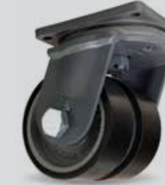
Maxi-Duty Dual Wheel (MDD) 5,000 – 15,600 lbs. Mounting Plate: 8-1/2" x 8-1/2"
