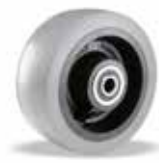
DuraGlide (95E) 1,600 – 8,100 lbs. A 1" thick ether-based poly runs cool under continuous, heavy loads to boost service life. High rebound provides excellent rollability for AGVs and tow-line carts.
