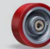
Press-On Poly (POY) 4,300 – 14,400 lbs. Extra-thick, extra wide urethane wheels for industrial trailers 5 tons and up. Solid tire chemically bonded to replaceable steel rim, pressed onto a cast-iron center.
