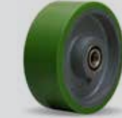
Duralast® (D) 475 – 9,000 lbs. Outwears rubber by 5-10 times. 95A liquid-cast polyurethane tread chemically bonded to a heavy-duty cast iron center. Non-marking; easy rolling.
