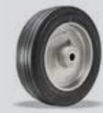
Super-Flex™ (SU) 300 - 1,200 lbs. Extra soft (60D), puncture-proof rubber tire vulcanized to a cast aluminum center delivers superior cushioning for outdoor use, like baggage trailers.
