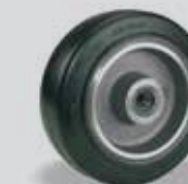
Press-On Rubber (POR) 2,800 – 9,300 lbs. With more cushion than poly tread, our highest capacity rubber wheel series curbs the effects of shock loading. Heavy-duty cast iron center with smooth tread.
