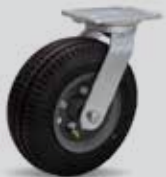
Heavy Duty Zinc (7100) 330 - 3,800 lbs. Pneumatic tire; heavy-duty forged steel, zinc plated swivel construction
