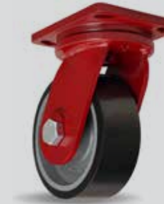
Enhanced Precision Super Duty (EPSD) 2,000 – 10,000 lbs. Mounting Plate: 6-1/2" x 7-1/2"
