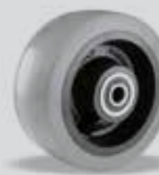
DuraGlide (95E) 1,600 - 8,100 lbs. The best poly choice for outdoor applications. Its 1" thick 95A hardness, ether-based poly resists the sun's UV rays, and won't break down under rugged, continuous use.
