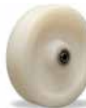
White Nylon (WN) 350 - 1,100 lbs. Nylon 6 resists water, solvents, and most chemicals and cleaning solutions. High capacity with exceptional abrasion resistance. Steam cleanable.
