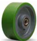
Duralast® (D) 475 - 9,000 lbs. Hamilton's classic 95A liquid-cast polyurethane tread chemically bonded to a heavy-duty cast iron center. Outwears rubber by 5-10 times. Wheel diameters up to 20".
