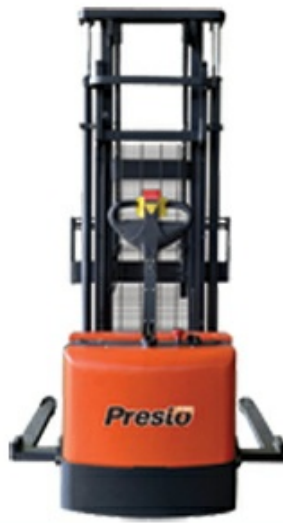
PPS3000-125AS $10,906 Telescoping Mast Straddle Stacker & Work Positioner
