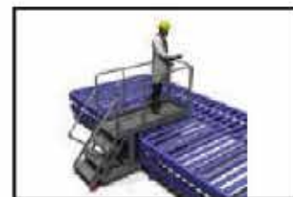
Conveyer Supported Cantilever Inspection Platform
