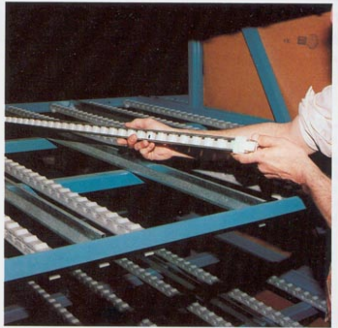
Kenrail track provides more wheels (on 1/2" centers) for better load distribution.
