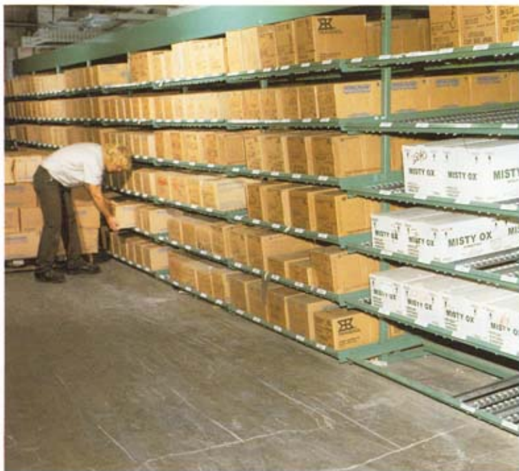
Picking full cases from Keneco system equipped with straight shelves.
