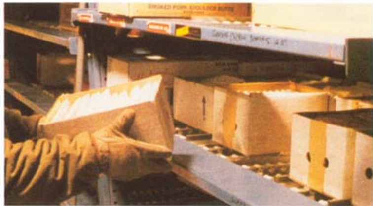
Impact tray at replenishment end protects track where heavy loads are used.
