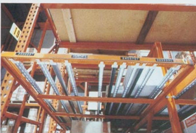
Shelf with gravity flow lanes is supported by pallet rack system. Keneco's ability to economically produce custom sizes which fit inside existing pallet racks results in material and space savings.
