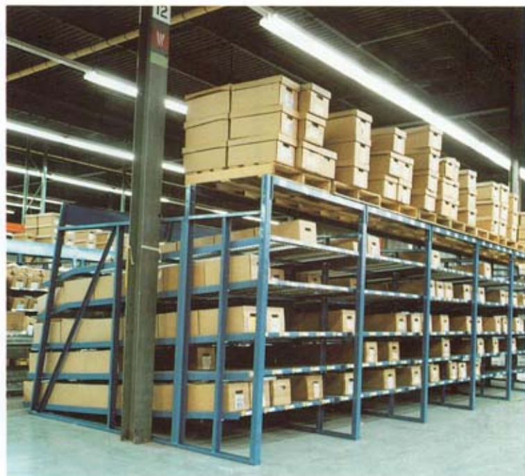
Restocking side of Keneco system. Single level pallet storage is provided above.
