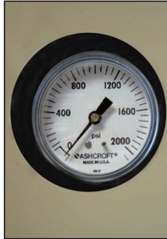
Clamping pressure can be adjusted by the user to prevent crushing of delicate loads.
