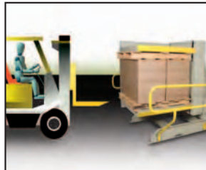
2. Place loaded pallet into rotator/inverter.
