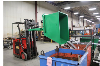
Step 3: Attachment and hopper design allow for 100% dumping capability.
