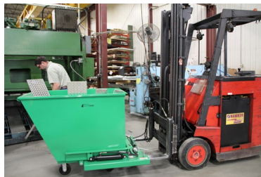
Step 2: Mobile hoppers easily and securely roll into attachment.
